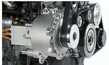
BSG 48V Mild Hybrids Dayco Accessory Drive & Aramid Cord Belts, Dual-art Tensioners, DDCS Crankshaft Decouplers
